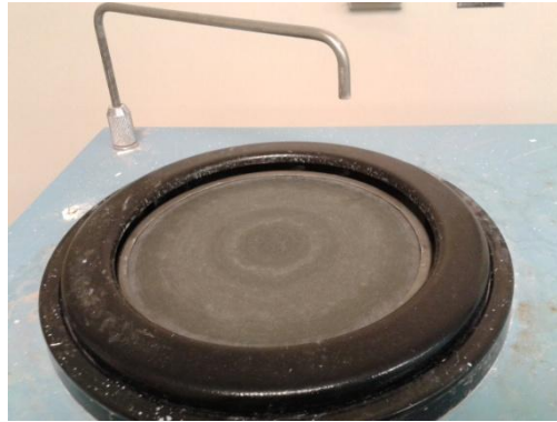
Fig. 2. Final set up of polishing wheel—ready to polish specimen
