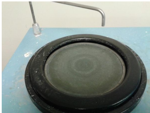
Fig. 6. Set up of polishing wheel—plastic splash guard in place.
