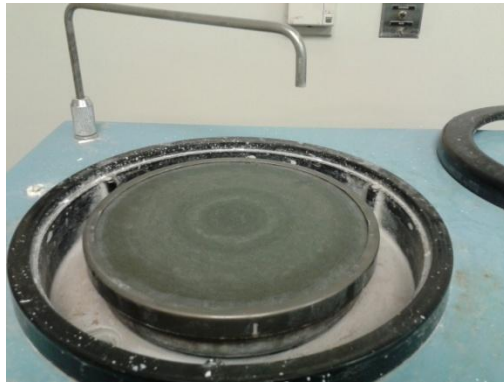
Fig. 5. Set up of polishing wheel—securing polishing medium to polishing wheel.
