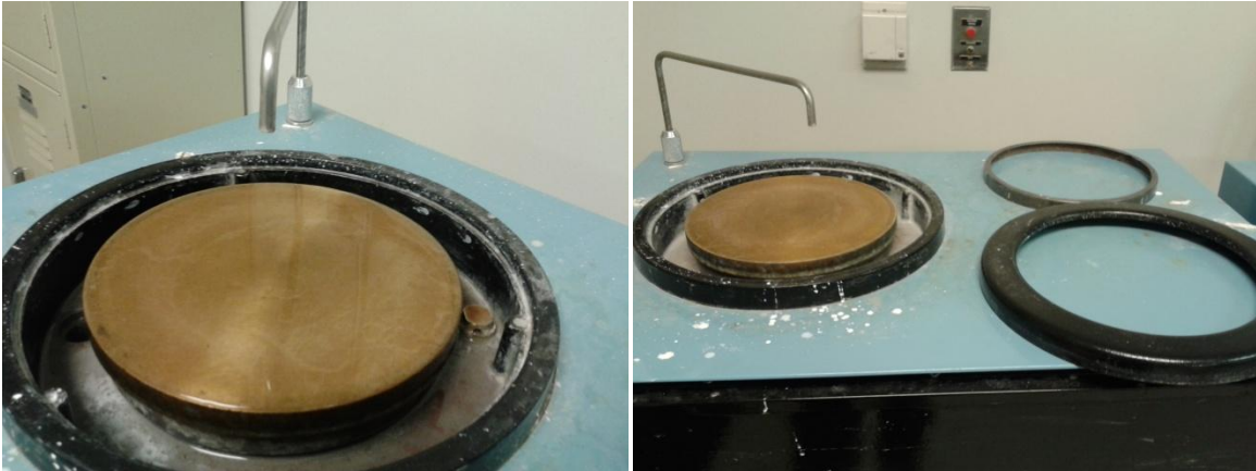
Fig. 9. Set up of polishing wheel—end of process.
