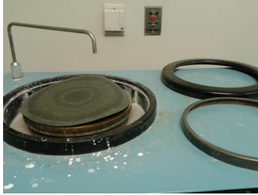
Fig. 4. Set up of polishing wheel—placement of polishing medium.
