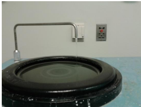
Fig. 7. Set up of polishing wheel—polishing wheel ready for use with water flowing from spigot.
